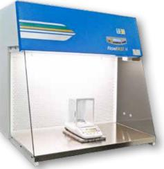
Faster FlowFAST H-RF is a safety workbench conceived for personnel and environment protection against powders and aerosol contamination.
